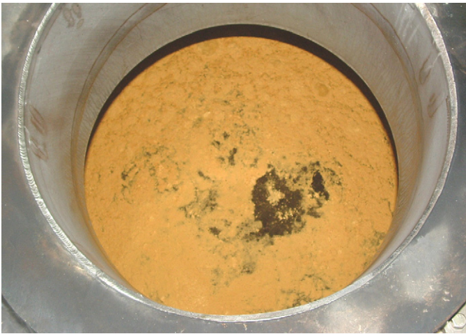
Fig. 3. Organic layer separated at the top of the SS tank in the plant.
